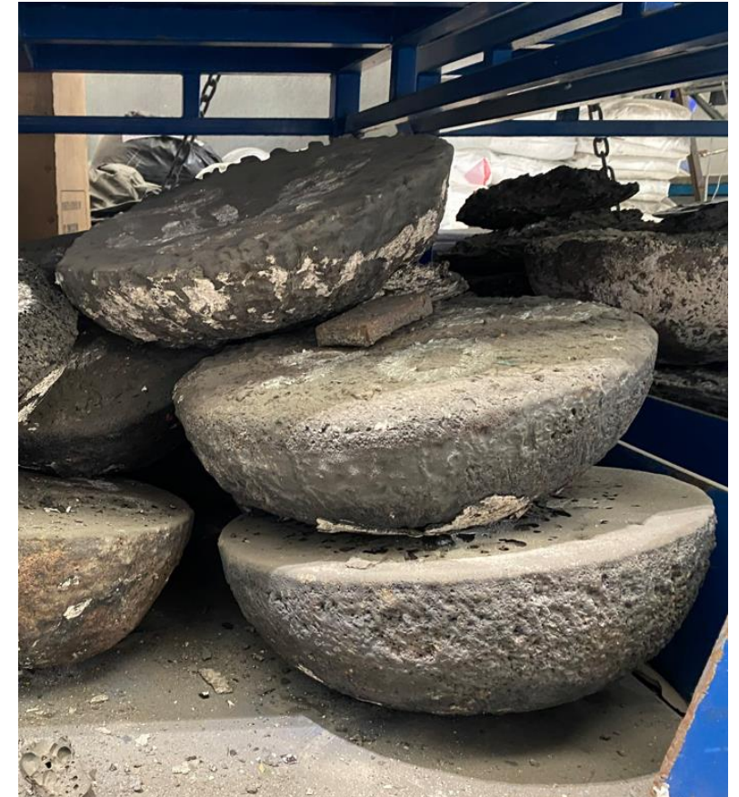
Smelter output: Copper alloy with trace elements (cobalt, nickel...) → hydrometallurgical treatment
