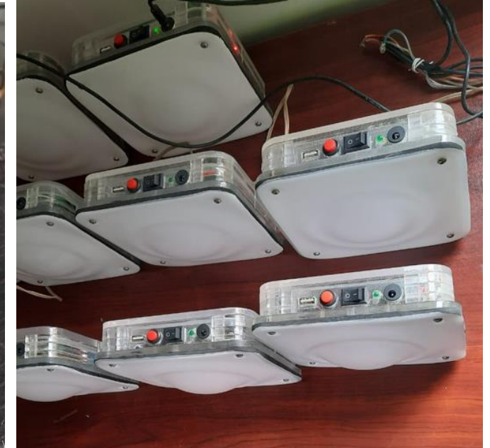
Rechargeable lanterns with second life battery cells
