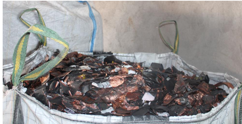
Copper foils and black mass from manual (!) Li-ion battery dismantling
