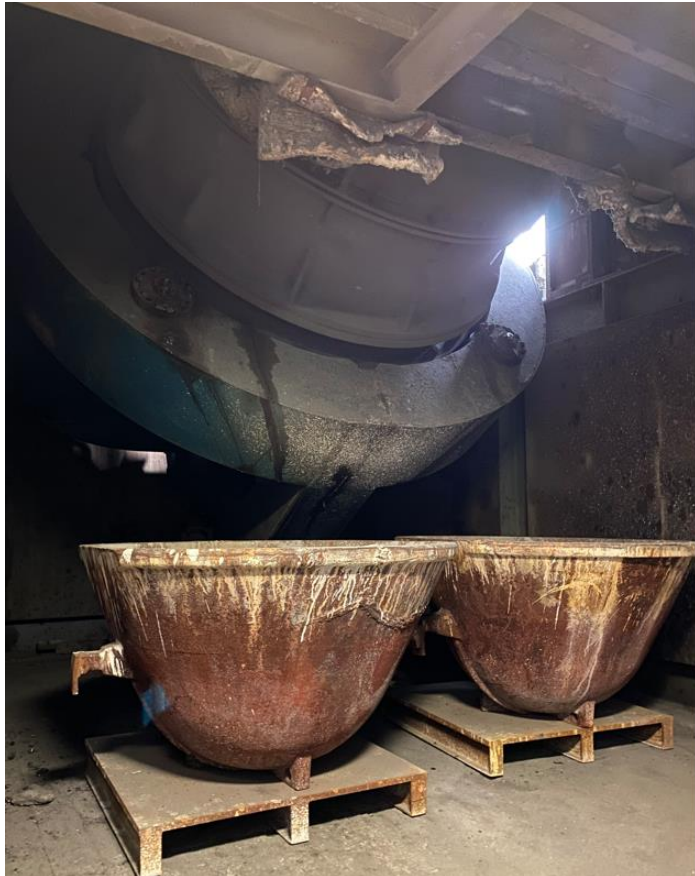
Battery cells & modules smelted in a furnace
