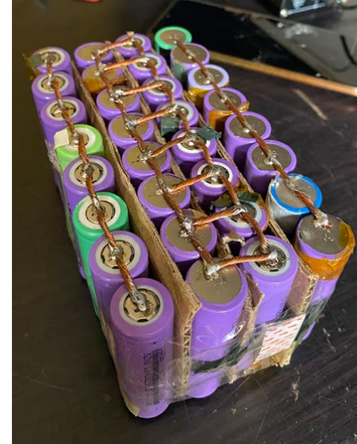
Battery from reused cells (sub-standard → unsafe products)
